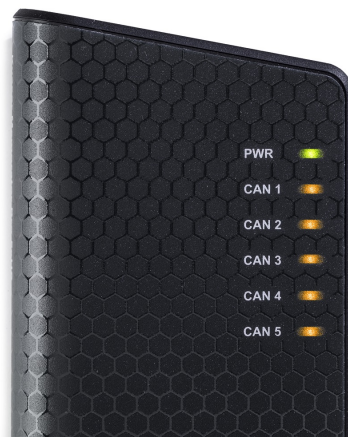
Figure 5: LEDs on the Kvaser Memorator Pro 5xHS.
