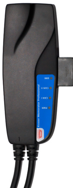
Figure 3: The CAN channels on Kvaser Memorator Professional.
