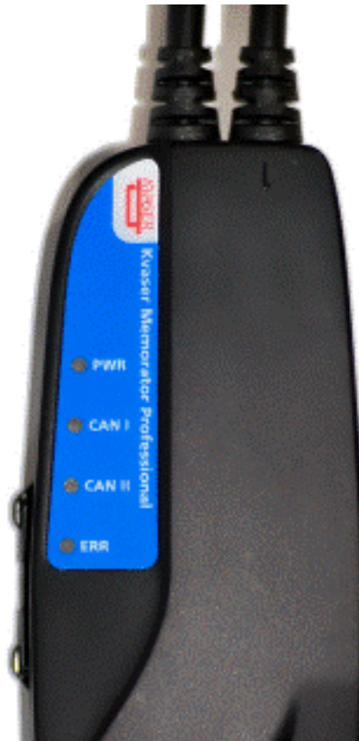
Figure 5: LEDs on the Kvaser Memorator Professional
