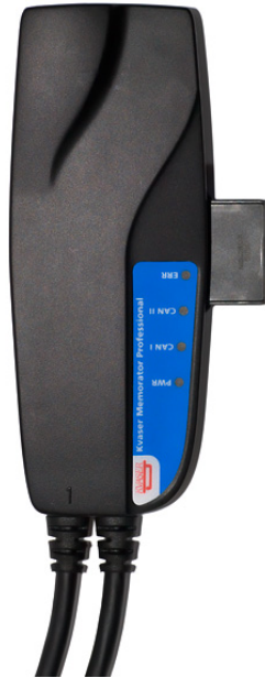
Figure 3: The CAN channels on Kvaser Memorator Professional.
