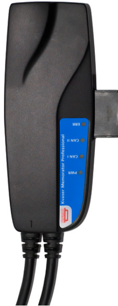
Figure 3: The CAN channels on Kvaser Memorator Professional.
