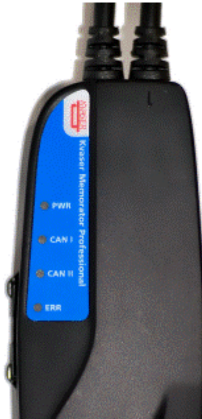
Figure 5: LEDs on the Kvaser Memorator Professional
