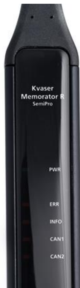
Figure 2: LEDs on the Kvaser Memorator R SemiPro
