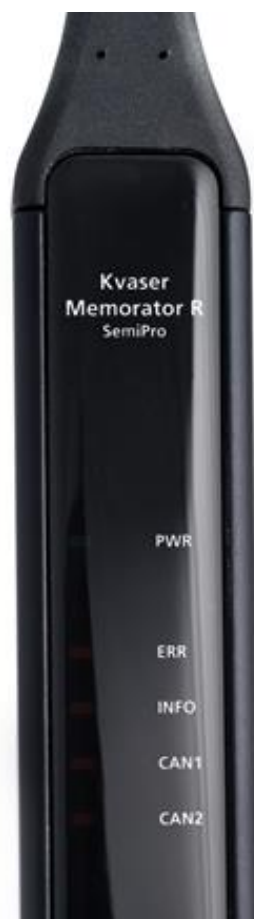
Figure 2: LEDs on the Kvaser Memorator R SemiPro
