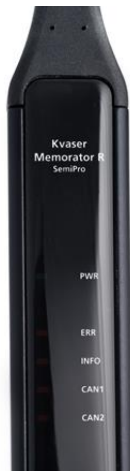
Figure 2: LEDs on the Kvaser Memorator R SemiPro
