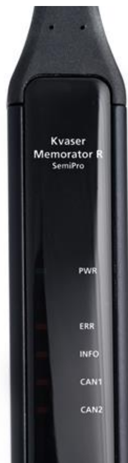
Figure 2: LEDs on the Kvaser Memorator R SemiPro
