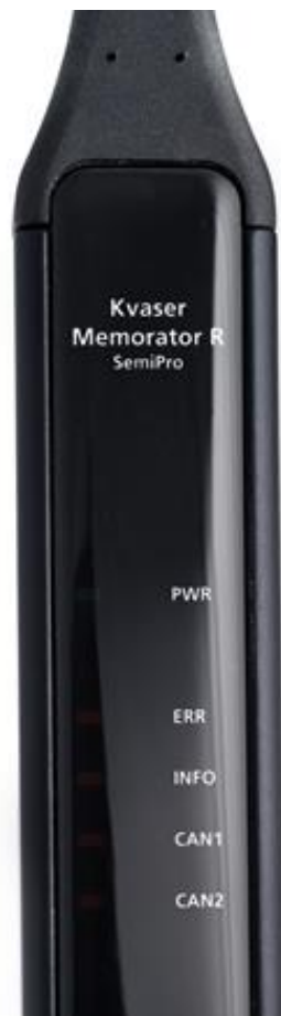
Figure 2: LEDs on the Kvaser Memorator R SemiPro
