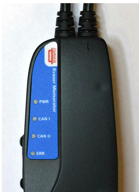
Figure 4: Kvaser Memorator LED indicators
