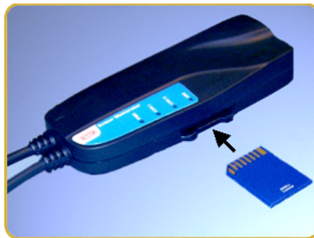
Figure 3: How to insert a memory card
