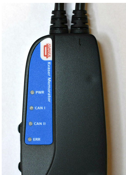
Figure 4: Kvaser Memorator LED indicators
