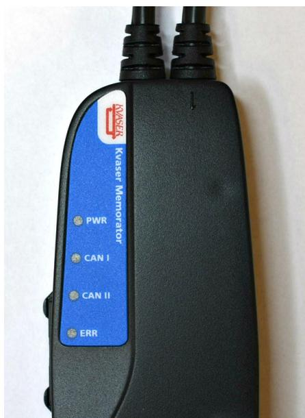
Figure 4: Kvaser Memorator LED indicators
