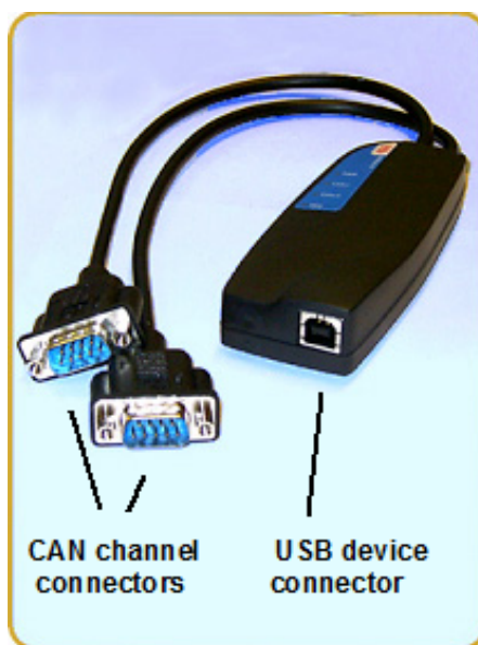
Figure 1: Connections on Kvaser Memorator
