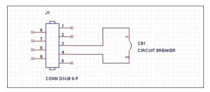
Figure 6: How to connect an external trigger switch
