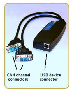
Figure 1: Connections on Kvaser Memorator
