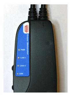
Figure 4: Kvaser Memorator LED indicators
