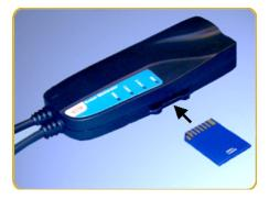
Figure 3: How to insert a memory card
