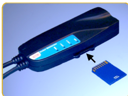
Figure 3: How to insert a memory card
