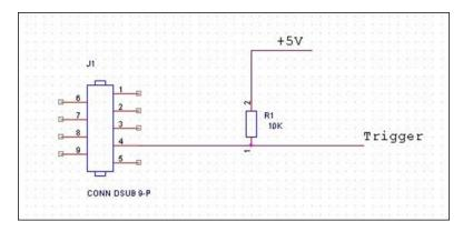
Figure 5: The trigger signal inside Kvaser Memorator
