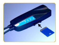
Figure 3: How to insert a memory card
