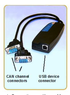
Figure 1: Connections on Kvaser Memorator
