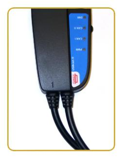
Figure 2: The channels on Kvaser Kvaser Memorator (channel 2 is not marked)
