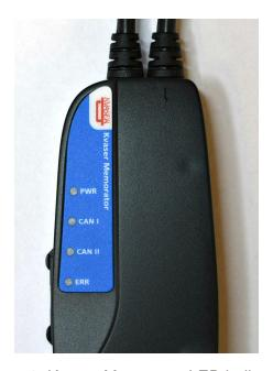
Figure 4: Kvaser Memorator LED indicators
