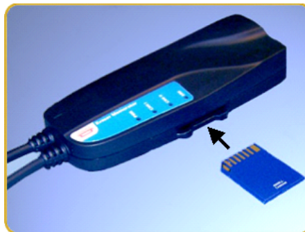
Figure 3: How to insert a memory card
