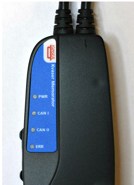
Figure 4: Kvaser Memorator LED indicators
