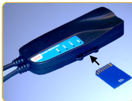
Figure 3: How to insert a memory card
