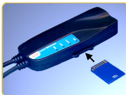
Figure 3: How to insert a memory card
