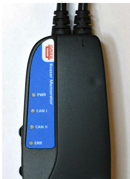
Figure 4: Kvaser Memorator LED indicators
