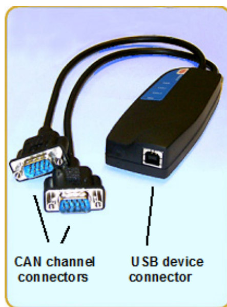
Figure 1: Connections on Kvaser Memorator
