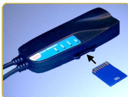
Figure 3: How to insert a memory card
