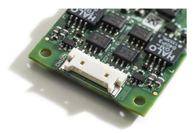
Figure 4: CAN connector on Kvaser Mini PCI Express 2xHS
