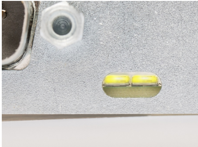
Figure 3: LEDs on the Kvaser PCIEcan 2xCAN v3.
