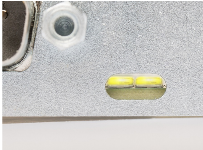
Figure 3: LEDs on the Kvaser PCIEcan 2xHS v2.
