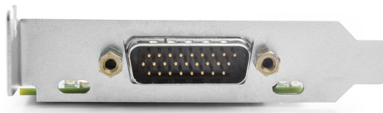
Figure 2: CAN connector on Kvaser PCIEcan 4xCAN v2
