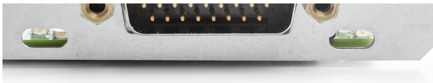
Figure 3: LEDs on the Kvaser PCIEcan 4xCAN v2.
