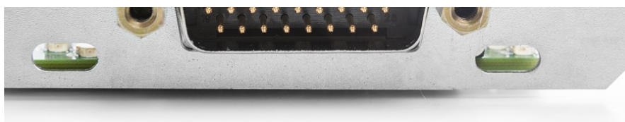
Figure 3: LEDs on the Kvaser PCIEcan 4xHS.
