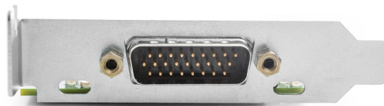
Figure 2: CAN connector on Kvaser PCIEcan 4xHS
