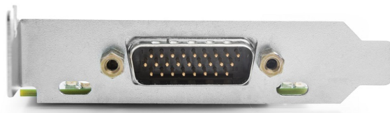
Figure 2: CAN connector on Kvaser PCIEcan 4xHS
