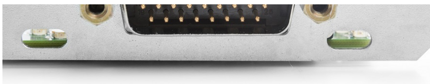
Figure 3: LEDs on the Kvaser PCIEcan 4xHS.
