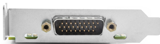
Figure 2: CAN connector on Kvaser PCIEcan 4xHS
