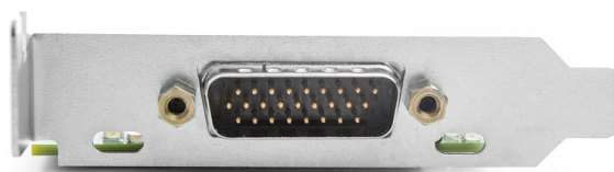
Figure 2: CAN connector on Kvaser PCIEcan 4xHS
