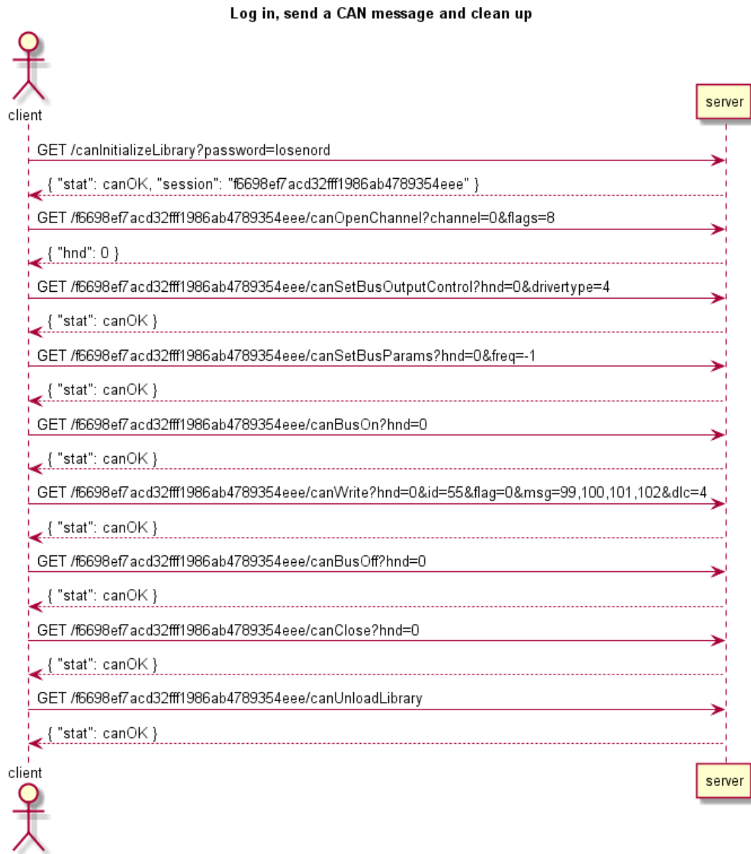
Figure 4: Log in, send a CAN message and clean up
