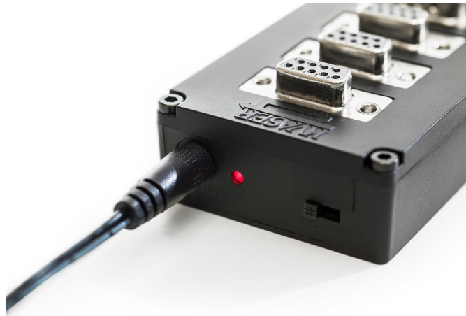
Figure 6: Power LED and termination three-way switch on Kvaser T-connector v2 (Base unit).
