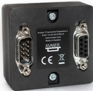
Figure 8: Bottom view of Kvaser T-connector L (Extension unit).
