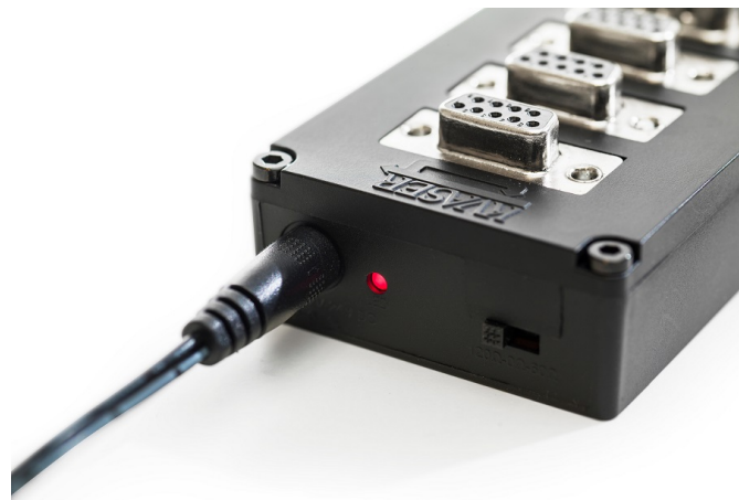
Figure 5: Power LED and termination three-way switch on Kvaser T-connector v2.
