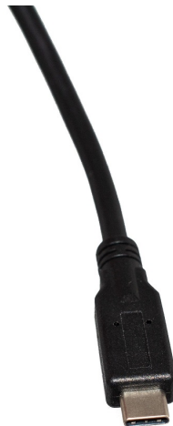
Figure 2: A standard USB Type-C connector.
