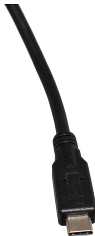
Figure 2: A standard USB Type-C connector.
