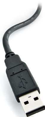
Figure 2: A standard USB type “A” connector.
