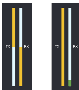
Figure 7: The yellow-lit area of the LED bars is proportional to the bus load. Both images indicate a bus load of 100%.
