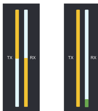
Figure 9: The total size of the LED Bars is proportional to the bus load. Both images indicate a bus load of 100%.
