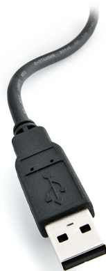
Figure 2: A standard USB type “A” connector.
