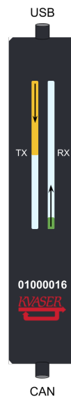
Figure 8: The TX LED bar lights up from the USB side to the CAN side of the unit, while the RX LED bar lights up from the CAN side to the USB side of the unit.
