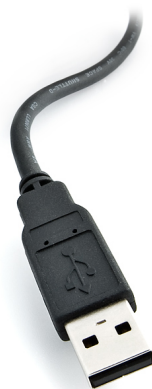
Figure 2: A standard USB type “A” connector.
