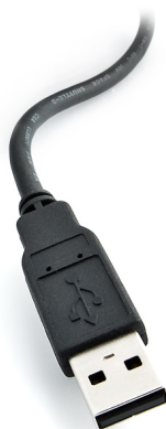
Figure 2: A standard USB type "A" connector.
