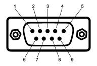
Figure 6: The male D-SUB 9 connector pin numbers
