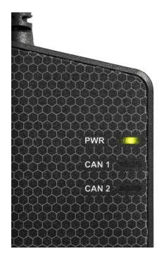
Figure 3: LEDs on the Kvaser USBcan Light.
