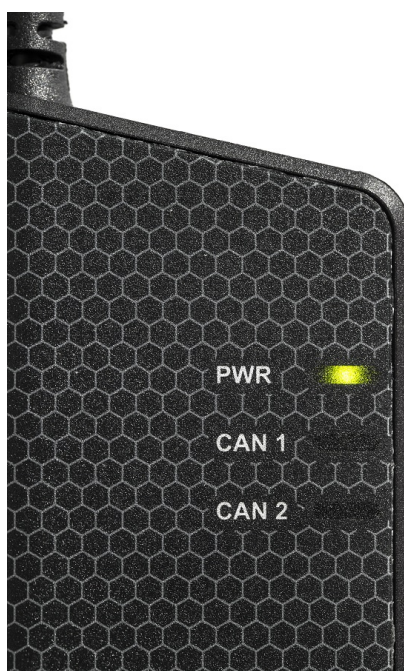
Figure 3: LEDs on the Kvaser USBcan Light.
