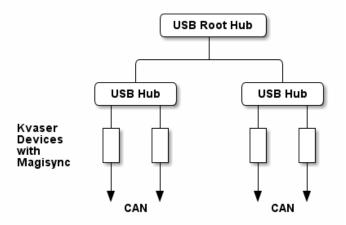
Figure 6: An example setup where all devices are synchronized via MagiSync.
